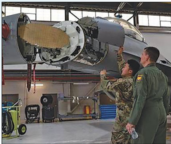
Figure 2 — An avionics specialist discusses an AESA radar installed in an F-16.
