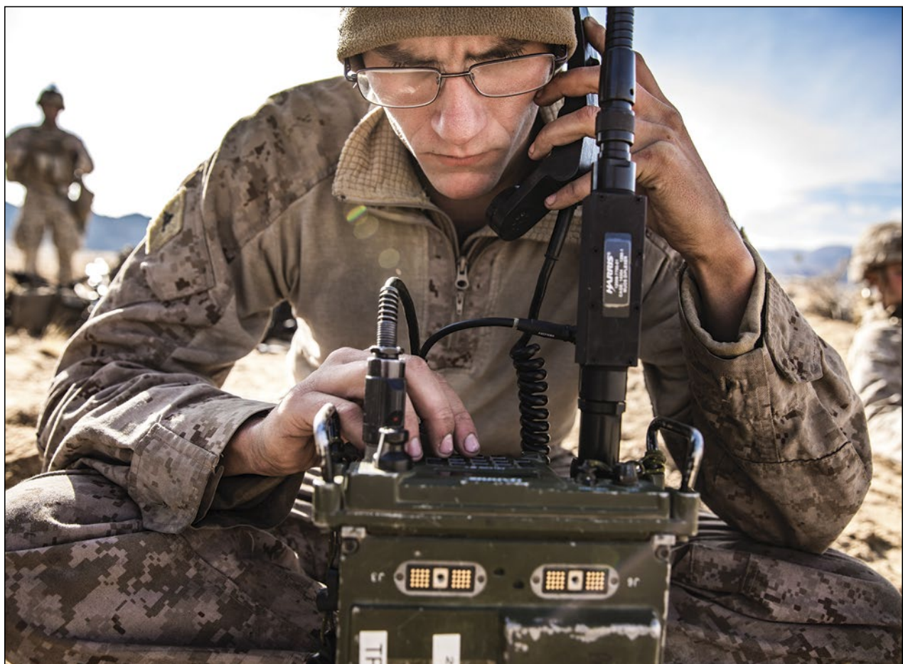
Figure 1 — A U.S. Marine Corps operator using an AN/PRC-117 multiband manpack radio during Exercise Steel Knight. Source: U.S. Marine Corps, public domain
